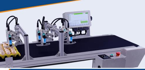
The entire pallet of eggs is transported through the conveyor belt. When the sensor detects the pallet signal, the relevant information is printed on the horizontal and hard rows of eggs in sequence to complete the batch coding and identification work of the entire pallet of eggs. According to the tray type or placement direction, you can freely select the number of print heads (maximum support 6 print heads) to adapt to various printing scenarios.
