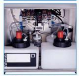
Double-head pump design makes more stable and durable. White ink machine has double mixing system to prevent the pigment ink precipitation.
